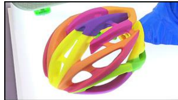
Objects 3D Printed on Stratasys "PolyJet" Material Jetting Hardware
