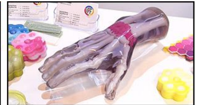
Objects 3D Printed on Stratasys "PolyJet" Material Jetting Hardware
